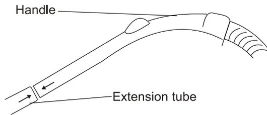
Insert the handle into the tube with a twisting force.
